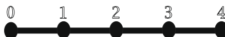
Fig. 2. Node 0 is on the boundary. In a fourth-order scheme, nodes 0–3 would be considered boundary points.
